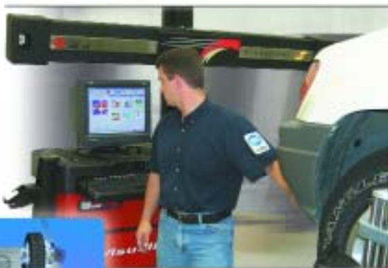
Computerized wheel alignment equipment sold by Myers prompts the operator through each step with continuous readings from eight sensors — creating the perfect alignment and reducing service time.
